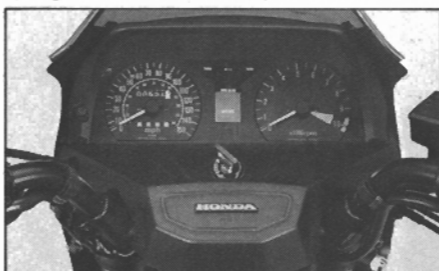
CB1100F's instrument panel includes 150-mph speedometer. Tubular handlebars fit into cast steel risers and are adjustable two ways.
